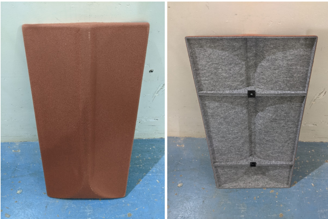
Figure 2 – Individual specimen panel; faces oriented away from (left) and toward (right) horizontal test surface
