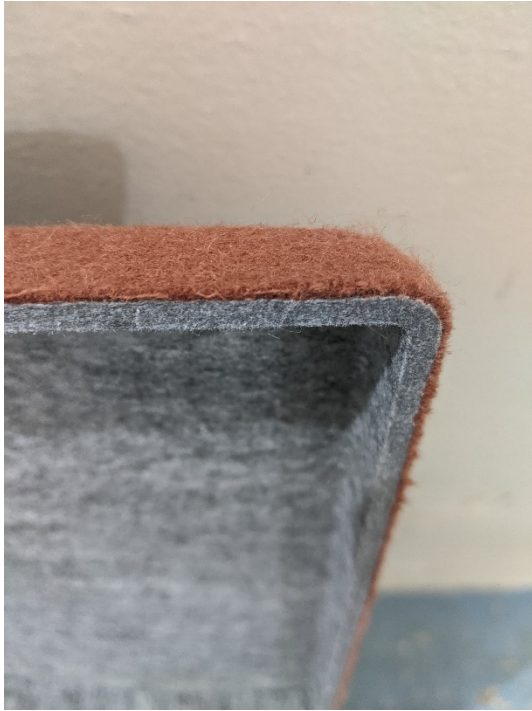
Figure 3 – Detail of felt shell and veneer material
